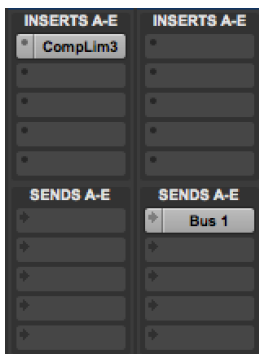
Channel Routing for Side Chain Compression
